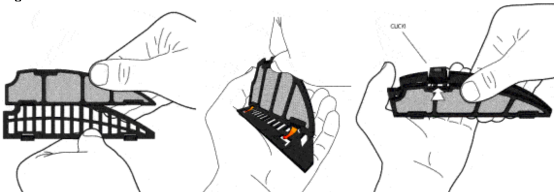
Figure 2a-c: Snap out old filter from Filter Door Frame (Figure 2a). Slide new Filter into grooves on Filter Door Frame (Figure 2b). Snap new Filter into Filter Door Frame as shown (Figure 2c).
